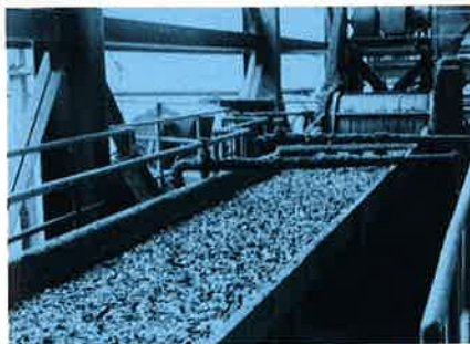
Fig. 63: Placing scrap metal on a rubber belt conveyor.
