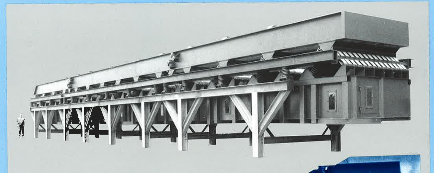
96" wide, 36" deep, 104' long, dust-tight trough design conveyor for distributing waste type fuels (RDF) to the metering bins of nine Boiler Feed Trains.
