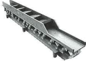
Fig. 35: This unit breaks up lumps as it conveys foundry sand.
