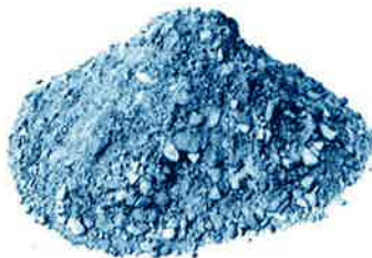
Fig. 4: A granular texture, usually with lumps, denotes a "General" kind of bulk solid.
