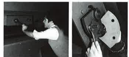
Fig. 46: If mechanical adjustments at "start-up" are needed, they are easy to do. The bolting of "turning plates" to the frame or adding eccentric weights to the motor are readily accomplished.
