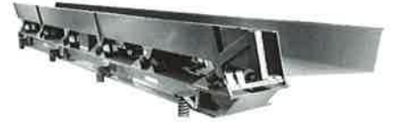
Fig. 40: A typical "Accumulating" Conveyor.
