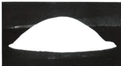
Fig. 3: "Floodable" bulk solids are very fine and dry.
