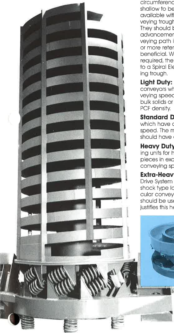
Fig. 47: A circular conveying trough.
