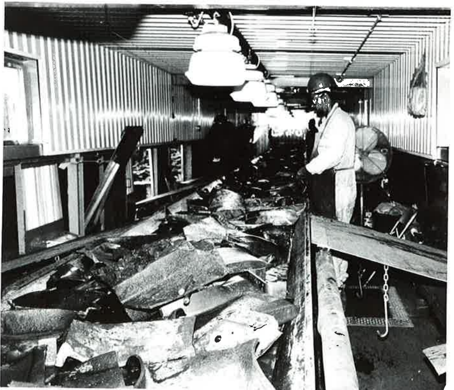
Fig. 59: Non-Ferrous Metal is being removed from this 48 in. wide by 98 ft. long "Picking and Sorting" Conveyor in a Recycling Facility. Requiring 3 HP, the Conveying Rate of the Scrap Metal is 50 TPH.
