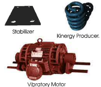
Fig. 13: The Kinergy Drive System has only three component parts. The steel coil drive spring that produces "Kinergy", the stabilizer to guide it, and the motor that supplies the needed heat energy to sustain the vibratory motion.
