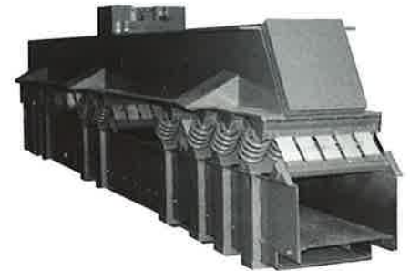
Fig. 25: The drive and the counterbalance are above the conveying trough. The unit's support is from its counterbalance.
