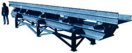
Fig. 22: A typical "counterbalanced" conveyor. Note the relatively light support structure which has the needed lateral truss members.
