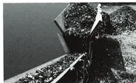
Fig. 63: Placing scrap metal on a rubber belt conveyor.
