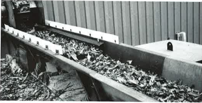
Fig. 55: Feeding wood scraps to a "hog" at a saw mill.
