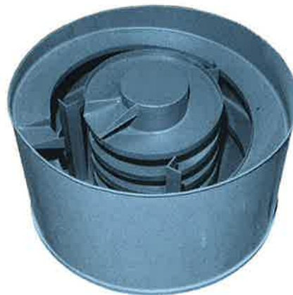
Fig. 32: A "Mixer" for bulk solids that utilizes circular conveying.
