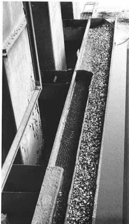
Fig. 51: Moving glass cullet with a multi-conveying trough unit. Note the "Imploded" liquid in the left trough section.
