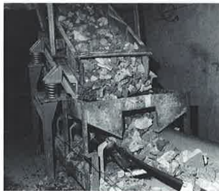
Fig. 62: Crushed rock being "reclaimed" from a storage pile above. The feeder is 36 inches wide by 7 feet long and it feeds 400 TPH, but only consumes 1.4 HP.
