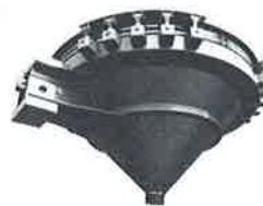
Fig. 15: The field follow of the Bin Activator instigated the formulation of the "Drive vs. Load" analysis in 1964. It could be applied to any vibratory machine, which included a vibrating feeder.
