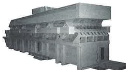
Fig. 30: The inlet of this feeder is kept full of "RDF" or wood waste such as bark, chips, shavings, or sawdust. As the fuel moves forward, it is subdivided into three feed streams that supply a "fluid bed" type combustor of a boiler.
