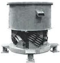
Fig. 18: A "unidirectional" feeder which conveys the material in a single direction.
