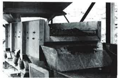
Fig. 65: This horizontal mounted feeder is 4 ft. wide by 12 ft. long. It has a screening deck to remove minus 1" size coal. The rate is 250 TPH and the power needed is 2 HP.
