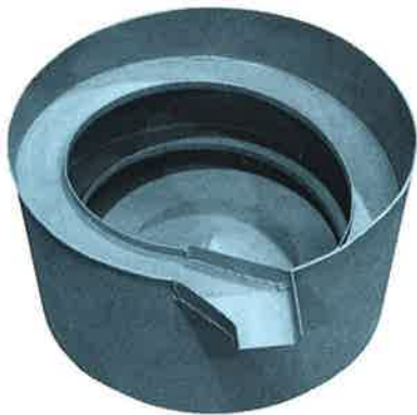
Fig. 53: Looking down on a circular feeder. The incoming material is received and stored in the center portion. It conveys in a circular path and gradually moves outward. By moving up the peripheral track, it is fed out near the top of the unit through a tangential discharge chute.
