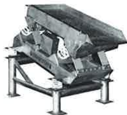
Fig. 9: Other functions, such as screening, can be performed while feeding.
