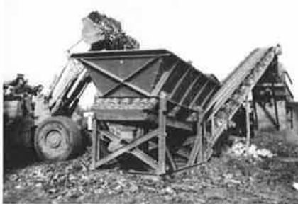
Fig. 67: Scrap metal being loaded into a feeder with an integral dump hopper. The unit uses 2 HP.
