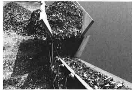
Fig. 70: This feeder with an integral dump hopper is discharging onto a belt conveyor that is feeding a shredder. The material is scrap steel, the rate is 250 TPH, and the needed input is 2 HP.
