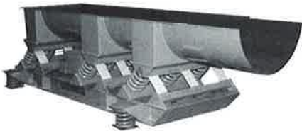
Fig. 18: A "unidirectional" feeder which conveys the material in a single direction.
