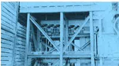
The Kinergy Driven Primary Crusher Feeder with a 5 HP input.
