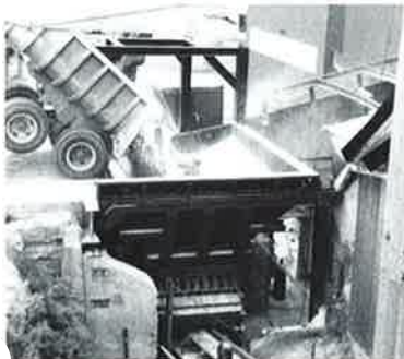
Fig. 40: Primary Crusher Feeders are one of the best examples of "load abuse" capability. The feeder is 5 ft. wide by 20 ft. long and it consumes 7.5 HP. The truck trailer is dumping 30 ton loads.
