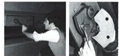
Fig. 52: If mechanical adjustments at "start-up" are needed, they are easy to do. The bolting of "tuning plates" to the counterbalance or adding eccentric weights to the motor is readily accomplished.
