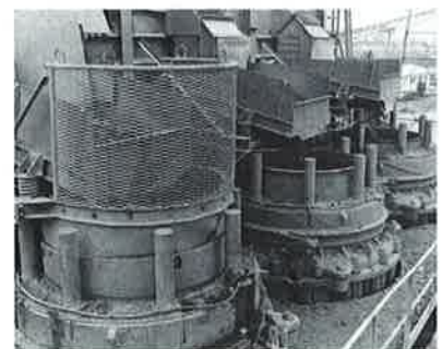
Fig. 49: Each of these three feeders supplies 800 TPH of minus 8" size limestone rock to secondary crushers in an aggregate plant. The power consumed per feeder is less than 2 HP! This "energy efficiency" reduces the "cost per ton" of rock produced.
