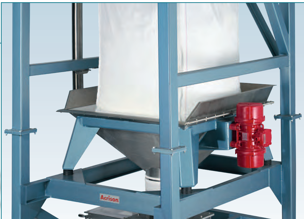
A close-up of a Model 810 Bulk Bag Unloader. The Unloader discharges into a slide gate, which is mounted above a volumetric feeder (not visible). The bag is nearly empty, lifted upward by a Bag Lifting Rack equipped with Acrison's optional Automatic Bag Tensioner (also not visible).
