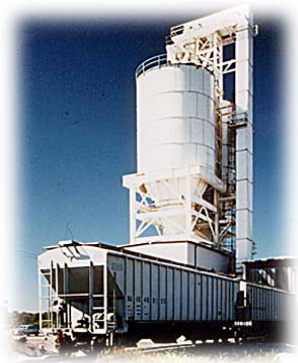
Model 0648-FSW-Z-90 handling 250 STPH of soda ash in rail-to-truck terminal
