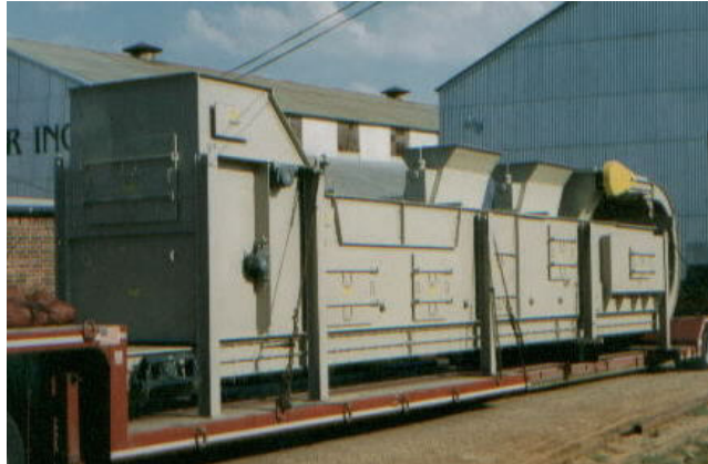
Lower horizontal casing with (2) inlets and Dribble-Drag™ clean-up conveyor
