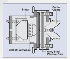
This produces a more powerful electromagnetic drive for higher stroke, larger capacity, and thus a smaller feeder than the competition.
