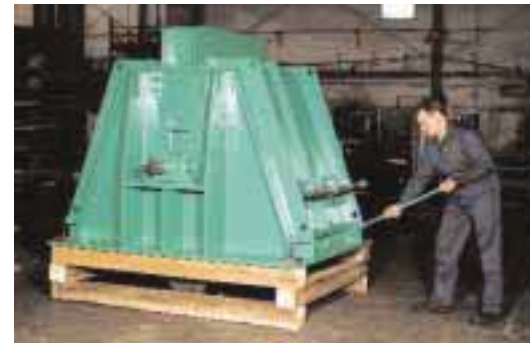
External adjustments are provided for adjusting the cage and for emptying the tramp iron pocket.
