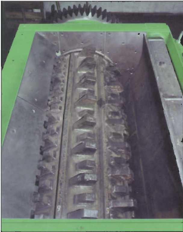
View from above; breaker plate is to the right
