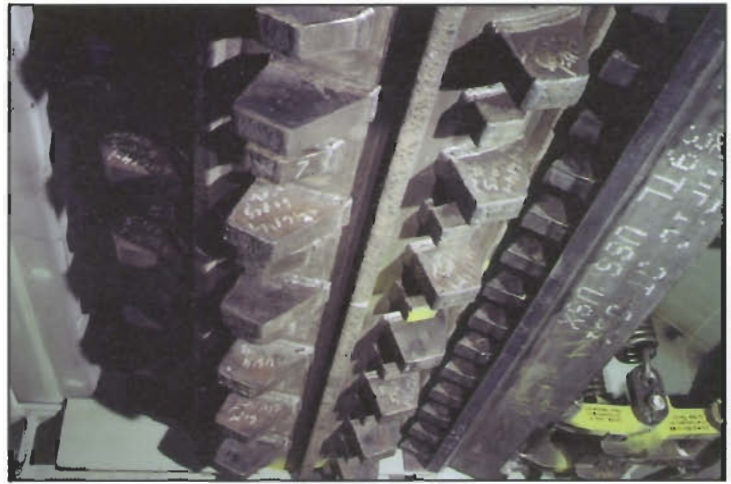
View from beneath. The lower lip of the breaker plate is immediately to the right of the roll. Behind that plate can be seen one of the two toggle release mechanisms.
