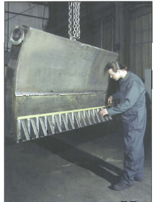
Every component and every subassembly, such as this breaker plate, undergoes numerous inspections.
