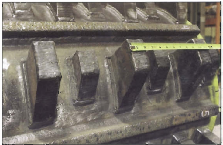
Teeth are welded to the roll shell, forming a very rugged and secure one-piece assembly.
