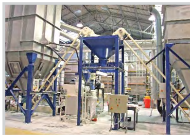
2 AMCs delivering tin oxide from process to packaging.
