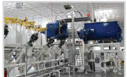
An AMC with multiple inlets delivering cement, sand, ash and recycled glass to a second unit that lifts them up into a mixer.
