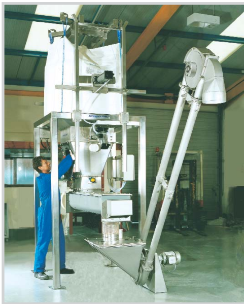
AMC designed for handling titanium dioxide. The aero mechanical conveyor is the only effective method of handling this type of product.
