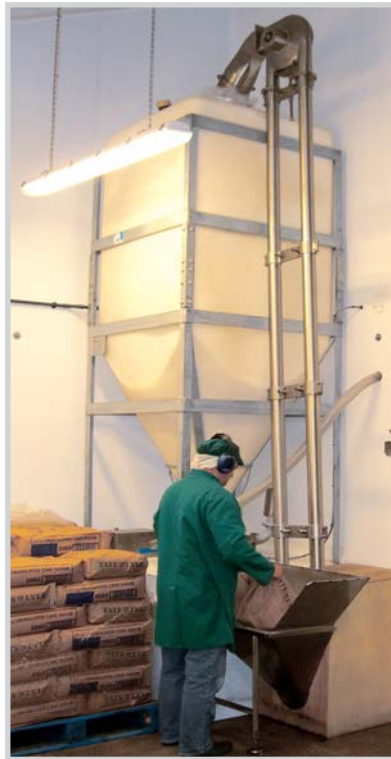
An AMC being used to unload sacks of sugar into a storage hopper.
