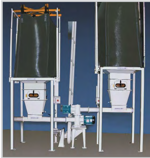
AMC elevating material from a transition hopper fed by two bulk bag dischargers via spiral conveyors.
