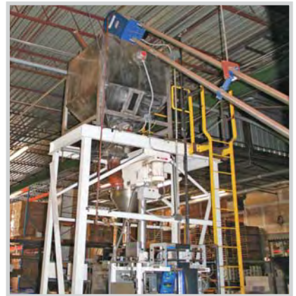
An AMC transferring flavored coffee powder from a blender up to a packing machine.
