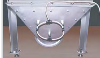
Inlet chute with aeration device.
