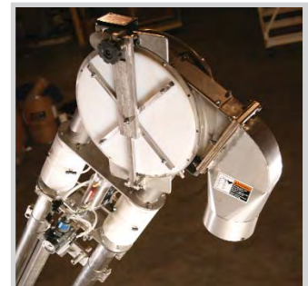
Automatic rope tensioner.
