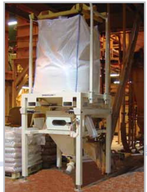
5. Bag loaded ready to discharge.
