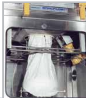
3. Pneumatic stretching device actuated to provide smooth path for product through spout and into downstream vessel, valve or conveyor.
