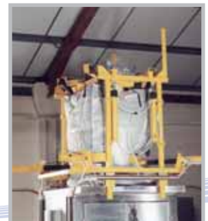
4. Bag Massagers at each corner assist flow and ensure total emptying.
