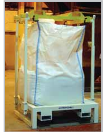
2. Loading bag into top frame.
