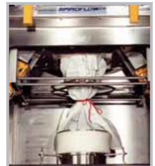
2. Spout pulled through the discharge dish (pinch bars open).
