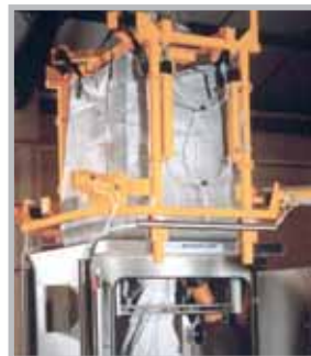
1. Bag is placed on discharger by hoist or forklift truck.
