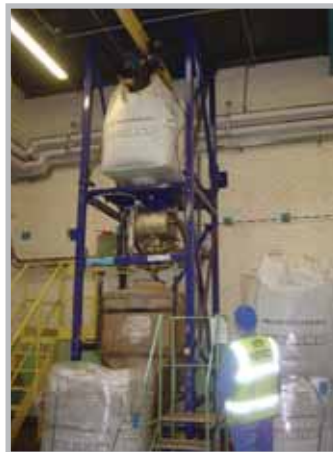
3. Traversing bag into position.
