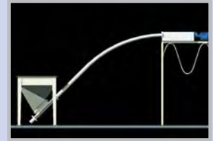
Horizontal outlet for restricted headroom.
