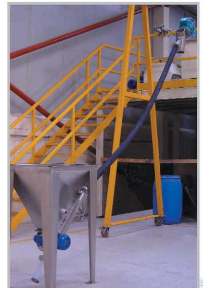
For heavy duty applications, our range of 'Megaflow' centerless conveyors is capable of throughputs of up to 40 tons/hr.
