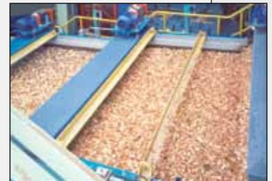
activated, the eccentricity of the shafts causes the bars to alternately rise and fall in a circular pattern. During the screening process, chips are repeatedly tipped and tumbled by the oscillating motion. Chips of acceptable size pass through the slots while overthick material is retained on the decks and carried over the end.
