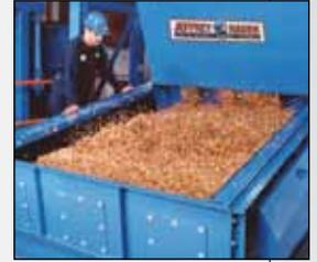
Optional features include adjustable inclination, and variable wave frequency.
