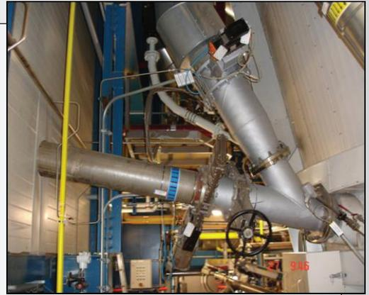
Our portable system is skid mounted with a hopper system for loading the material. A twin screw will feed the material either directly into a pneumatic system or on to a weigh belt feeder (when greater accuracy is required). The material is then blown directly into a boiler, kiln or discharged through a cyclone (when mechanical feed is used).
