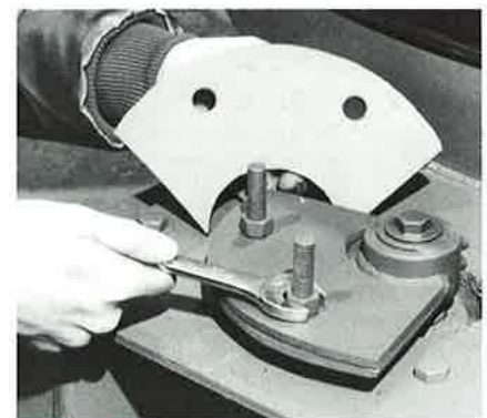
Fig. 19: Easy adjustment of the eccentric weights.
