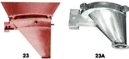
Fig. 23: This eccentric unit induces wood chips to flow from a bin. The pipes on the side wall are inlets for steam which help to pre-condition the chips for digestor downstream.
