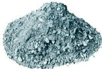
Fig. 3: A granular texture, usually with lumps, denotes a "General" type bulk solid.
