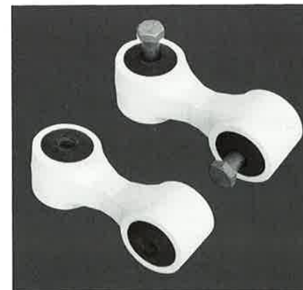
Fig. 11: The 90° twist and the large rubber bushing make this hanger arm the best available.
