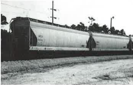
Enclosed cars with smooth surfaces and curved side walls. Courtesy, ACF Industries, St. Charles, Mo.
