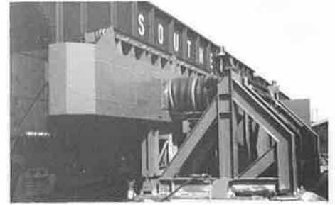
Less than 8 HP is needed to unload this 100 ton car. Evaluating its "RMS" (root-mean-square) power consumption reduces it to only 1.75 HP. That's being "energy efficient"!
