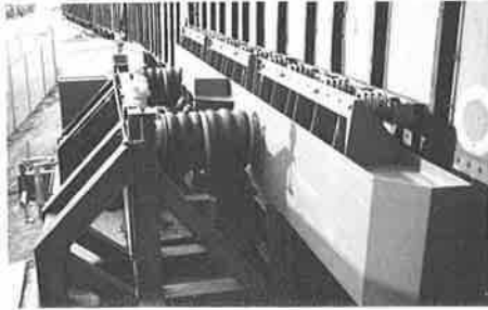
Full length, thick rubber bumpered attenuators are now used to restrain excessive movement in the upper part of the car's side wall. This helps to quiet the rail car as it approaches being "empty."
