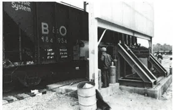
In 1980, the first Discharger for unloading coal at a power plant went into service. The overview on the left shows the simplicity of the unloading station. Located in Plymouth, N.C., this Discharger of early design vintage is still in productive use.
