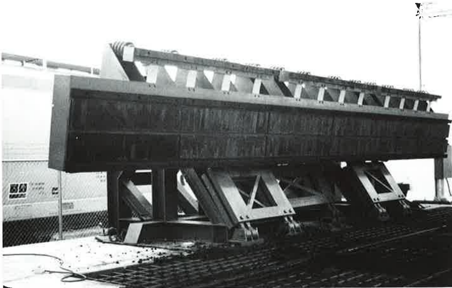
Terminals usually need fast unloading of 100 ton cars. To accomplish it, this unit has a car contacting member that is 32 ft. long so it can fully engage both end slopes.
