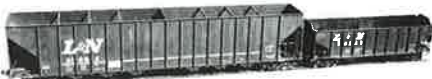
Car lengths can vary from 28 ft. (50 ton) to almost 70 ft. (7,000 cu. ft.) as shown by the large wood chip carrying car on the left. Courtesy Ortner Freight Car Company, Milford, Ohio.
