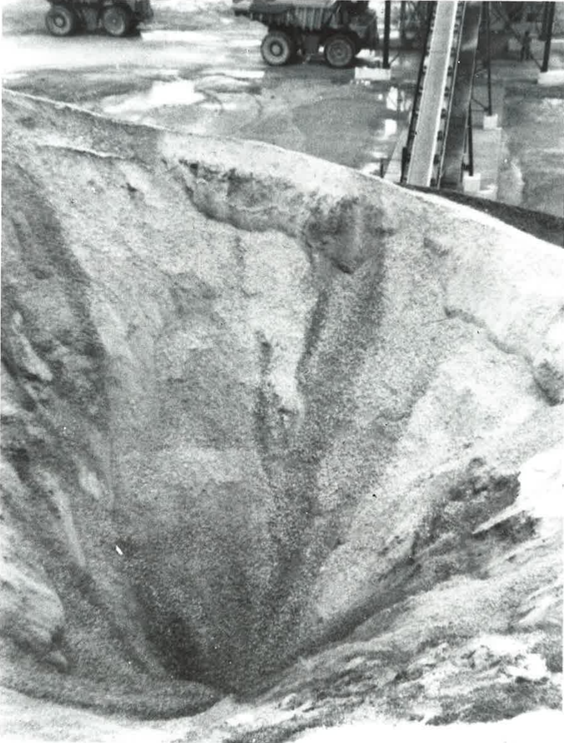
Fig. 14: Looking down into the crater of Expanded Flow. Both the size of the pile and the recent rain can be related by noting the trucks and the ground level water puddles standing in the top of photo. When the upper layers of the pile freeze, the desired Expanded Flow pattern will still be achieved. Note: The Storage Pile Discharger cannot be seen because it is buried under the pile of limestone; however, its effect on the pile is clearly visible!
