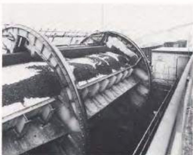
The major application for Pennsylvania Frozen Coal Crackers is under rotary car dumps. This is the point where most frozen coal problems can be solved.
