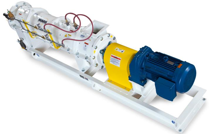
The material enters at one end of the cylinder and is whipped by the pins as it moves from the inlet, through the shell and to the bottom outlet. As a fine spray of liquid is added at the entry section and distributed throughout the powder, fine mixing and micro-agglomeration will occur. The end result is a wetted, agglomerated and densified micro-pellet.
