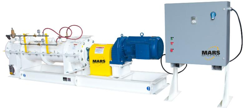
The material enters at one end of the cylinder and is whipped by the pins as it moves from the inlet, through the shell and to the bottom outlet. As a fine spray of liquid is added at the entry section and distributed throughout the powder, fine mixing and micro-agglomeration will occur. The end result is a wetted, agglomerated and densified micro-pellet.
