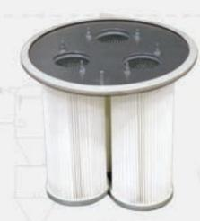
The filtered air flow is momentarily halted, and the Filter Media is firmly flexed causing accumulated dust particles to drop from between the pleats into the hopper below.
