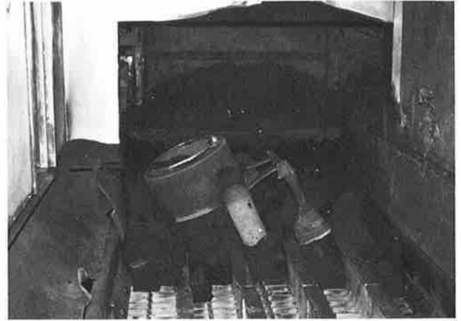
Fig. 16. This 60-in. wide by 42-ft. long sand cooler needs only 10 HP. The adjustable conveying speed is a true benefit.
