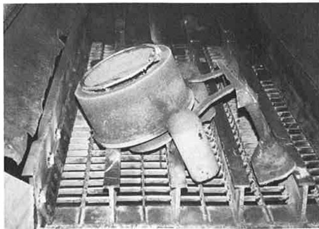
Fig. 17. Continuous shakeout feeders have been improved by the use of the kinergy drive system. Longer lengths are now practical, and the easy change in stroke and frequency for preventing casting damage is a real advantage.
